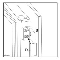
If the appliance is fixed to the side of the kitchen unit, simply slacken the screws in the fixing brackets (D), move the brackets as shown in the figure and re-tighten the screws. Then fit cover (E).
